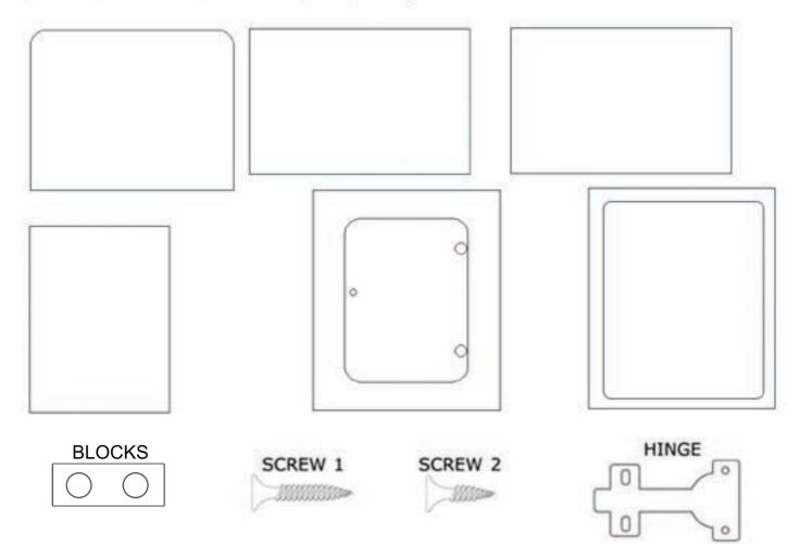
Fasten blocks to sides and top & bottom of front & rear panel and top and bottom of side panels, using screw 1.
