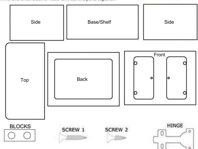
Fasten blocks to sides and top & bottom of front & rear panel and top and bottom of side panels, using screw 1.
